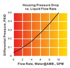
\* For liquids other than water, multiply the pressure drop by the specific gravity of the fluid.
